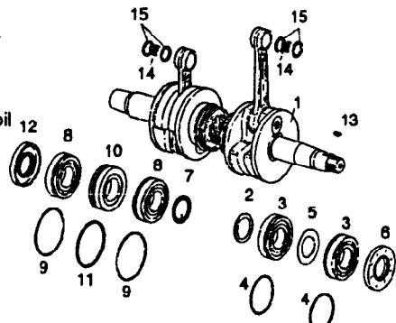
Will be replaced by the new crankshaft with the Rotax part number 887 051 crankshaft assy, Items 1-15 (complete with outer bearings, woodruff key, oil seals and piston pin bearings).
