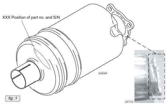
Inspect area for exterior traces of smoke and for cracks!
