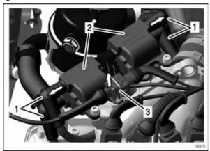
1 Ignition coil connector2 Double ignition coils3 EGT-connector
