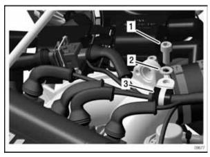
1 M6x14 Allen screw 2 6.4 washer 3 cable clamp
