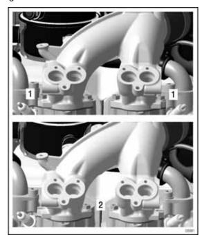
1 Outer screw-fastening 2 Inner screw-fastening
