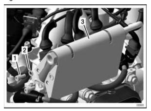
1 M5x12 Allen screw 2 washer 5.3 3 Heat shield
