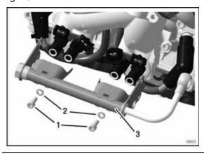
1 M5x12 Allen screw 2 Lock washer DIN 128-A5-FST 3 Fuel rail
