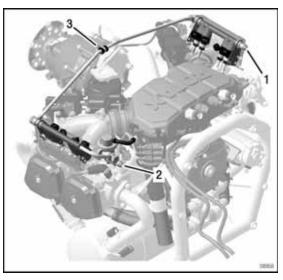
1 Fuel rail 1/3 feed line 2 Fuel rail 2/4 outlet line 3 M6x16 Allen screw
