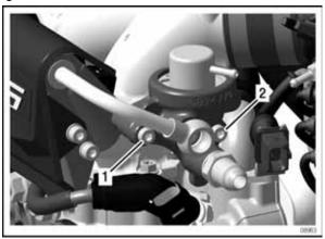
1 M5x35 Allen screw 2 M5x45 Allen screw
