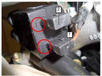
1 Ignition coil connector (red cable) Plus (+) 2 Ignition coil connector (black cable) Minus (-) 3 Double ignition coil
