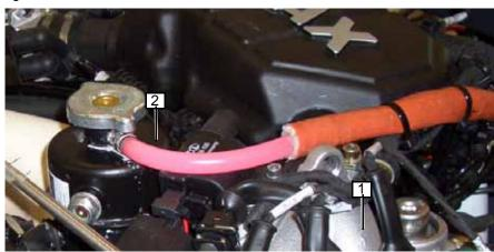
1 Intake manifolds2 Expansions tank
