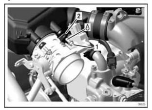
1 Hex./Torx-flange screw M6x16 2 Separating plate
