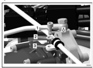
1 M6x16 Allen screw 2 Washer 6.4 3 Cable clamp 8/M6
