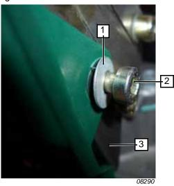
1 Spring washer 12x5.2x0.5 2 M5x12 Allen screw 3 Heat shield
