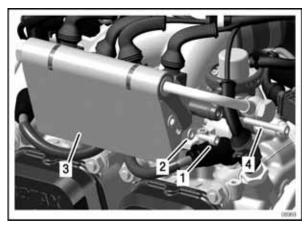
1 M5x12 Allen screw 2 5.3 washer 3 Heat shield 4 M5x35 Allen screw
