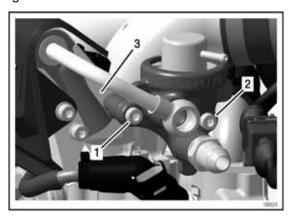
1 M5x35 Allen screw 2 M5x45 Allen screw 3 Heat shield
