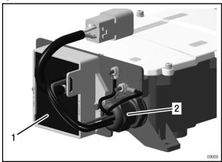
1 Regulator B 2 Cap nut of the gasket screw connection
