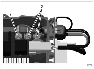
1 Lock nut M5 with washer 2 Lock nut M4 with washer
