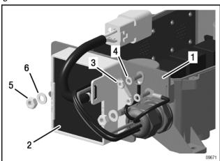
1 Regulator plate 2 Regulator B 3 Lock nut M4 4 Washer 4.3 5 Lock nut M6 6 Washer 6.4
