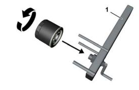
1) Oil filter cutting tool part no. 276270
